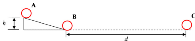
Fig. 2. A schematic showing a test material in a rolling resistance measurement.
