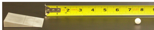
Fig. 3. A photograph showing the simple setup for measuring CoRR of a Teflon ball using a ramp of height h and measuring the distance traveled on a flat substrate d .
